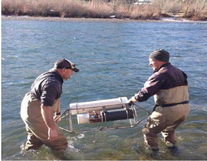
Figure 3: SAMI-alk being deployed in the Clark Fork River in November 2016. Field tests are continuing during 2017.
